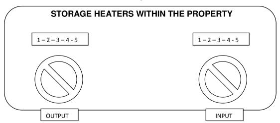
The storage heaters are connected to the "Off Peak Supply" This supply is only active overnight i.e. between 12 midnight and 07:00am and is switched on and off via either a time clock or teleswitch the cost for this is approximately 50% of the normal rate charged for the electricity for the rest of the house.
